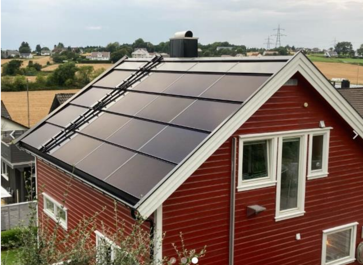
Silk® Nova Red 370 Wp 108 CELLS HALF-CUT – MULTI BUSBAR
